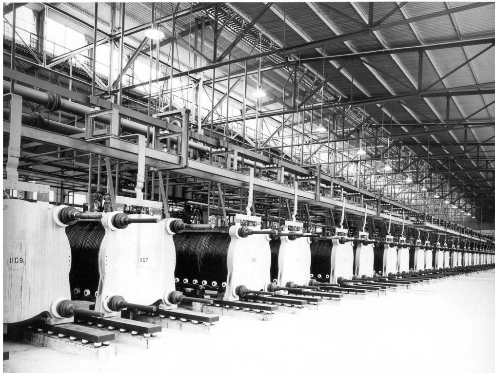
Norsk Hydro's 30,000 Nm 3 /h (~150 MW) Electrolyzer Plant (1948 - 1990)
